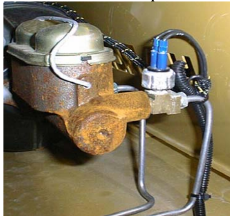
Master Cyl. with Brake line installed
